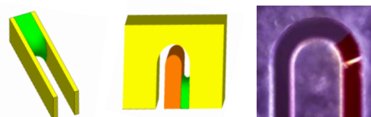
Figure 3 : Sketch of a suspended capillary flow between two vertical plates and in a winding channel; on the right, whole blood capillary flow in a winding suspended channel.
