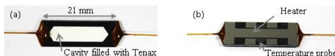
Figure 1 : Example of Si micro-preconcentrator chip filled with Tenax. (a) Front side, (b) back side.
