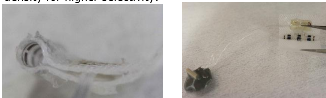
Figure 1 : left: Silicone cuff with embedded parylene electrodes and electrical wire. Right: Cuff fully packaged with electrical connector
