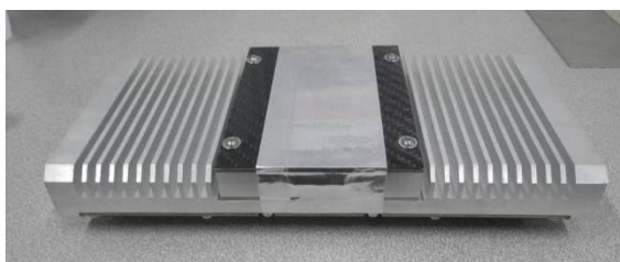
Figure 3 : ME100 linear array pixel detector [3]
