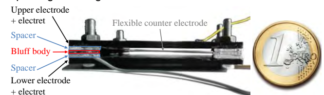
Figure 2. Electret-based electrostatic flutter energy harvester [2, 3].
